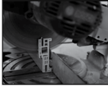
Bước 2: Cắt 2 gờ khung bao đứng Step 2: Cut the vertical frame edges as the technique drawing.
